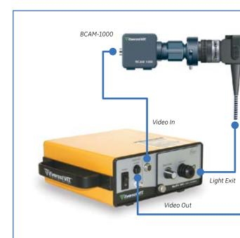
Fiberscope camera system usii
